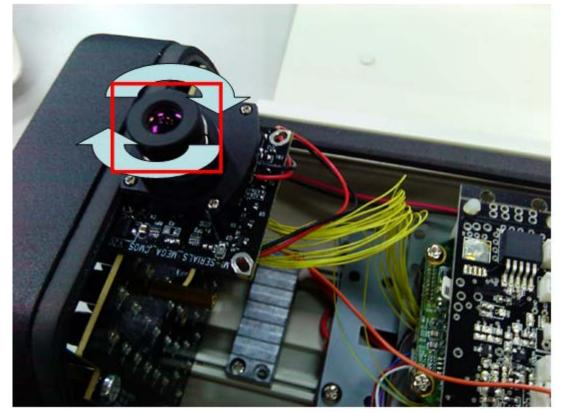
Step5. Take of the lens, and set the focus by turning the lens to the left or right direction.
