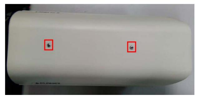
**Step3.** Turnover ICA-HM350, and you will see the two screw, use screw driver to loose the two screw on ICA-HM350 plate.
